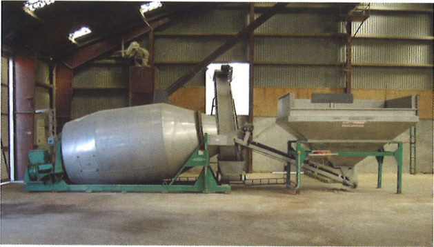
Figure 2. Shamrock blender 9 t per batch to blend with a capacity of 50 tph.
