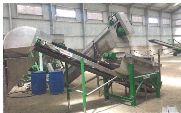
Figure 5. Fertilizer screen line to remove bigger particles out of the fertilizers.
