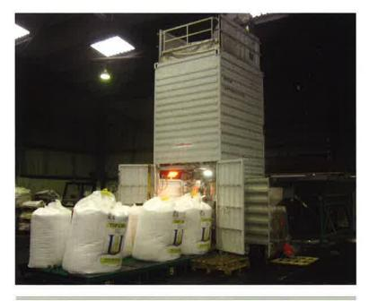
**Figure 5.** Warehouse storage, EMT 20 ft vertical container big bag line 140 tph.
