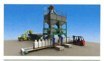
Figure 3. 3D CAD representation of a big bag line and blender.
