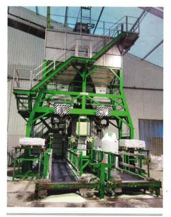
Figure 1. EMT high-speed big bag twin line 140 tph.
