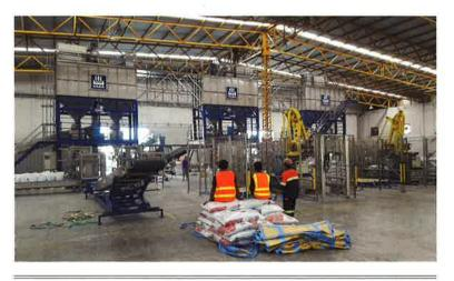
**Figure 4.** EMT small bags filling line with a total handling capacity of 240 tph, installed for a customer in Thailand.
