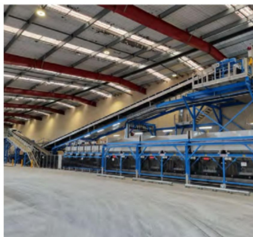
Figure 1. 17-hopper weighing continuous blender.
