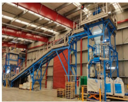
Figure 2. Big bag line capacity of 80 tph.
