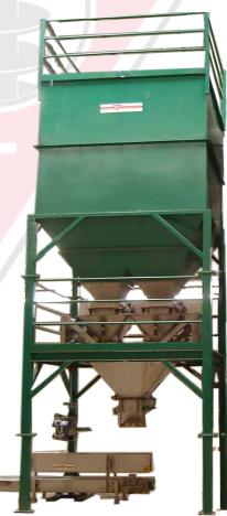
The Small Bag Double Unit is an automatic bag fill system for 15 to 50 kg bags. This machine is suitable for powder and granular materials.
