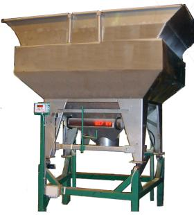
The Smithbuilt open top blender is suitable for granular fertilizer production. The machine processes all raw materials into an excellent blend. When the machine has produced a blend it can be transported to a bag
