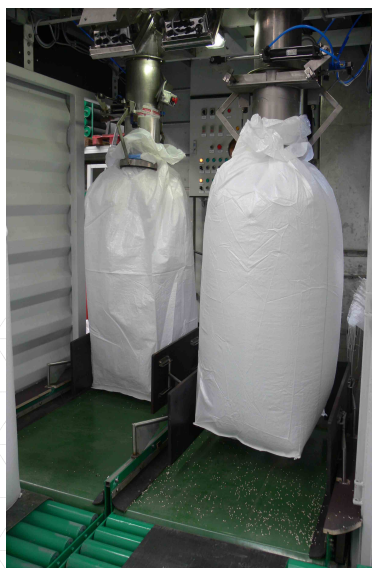
FILLING OF BIG BAGS INSIDE THE CONTAINER
