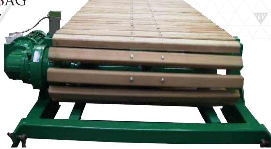
The big bag Conveyor is a horizontal This bag is closed at the same time as a wooden chain conveyor that transports FIBC (Flexible, Intermediar, Bulk, Con- The Conveyor can move 1000 kg big tainers) bags.
