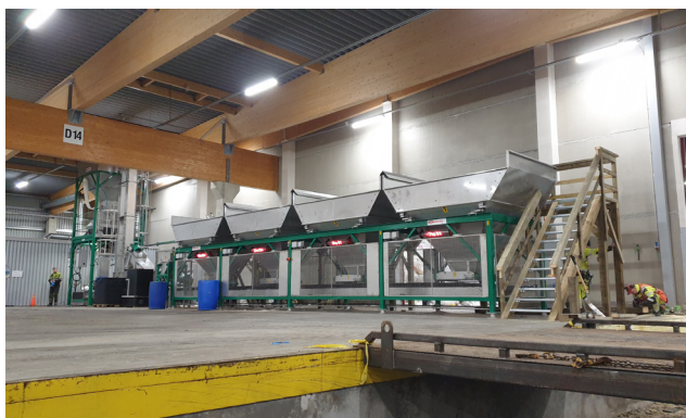
Figure 6. Continuous Weighcont type blender in the fertilizer warehouse of Cemagro, Finland.
