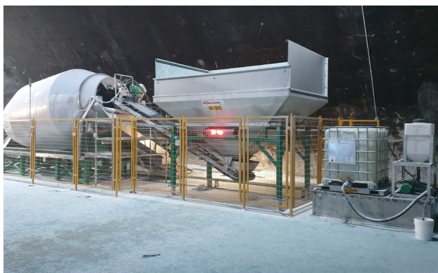
Figure 7. Typical setup of a Shamrock type batch blender with intake hopper and liquid adding unit.
