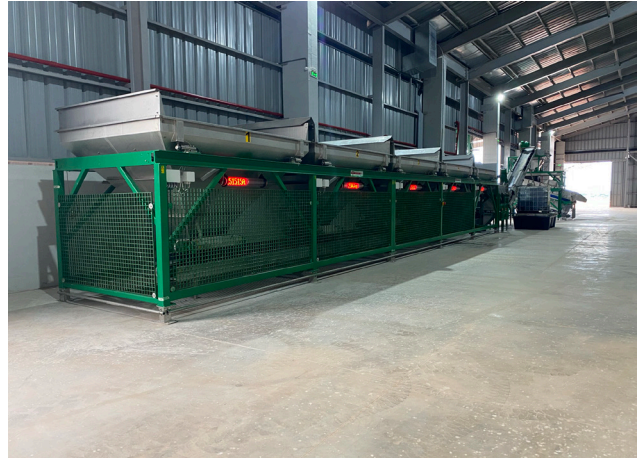
Figure 4. Continuous Weighcont type blender line with weighing hoppers and liquid adding to bagging units.
