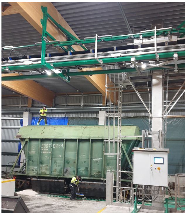
Figure 5. Train wagon discharge in a pit and elevator to warehouse filling conveyor installed at Cemagro, Finland.
