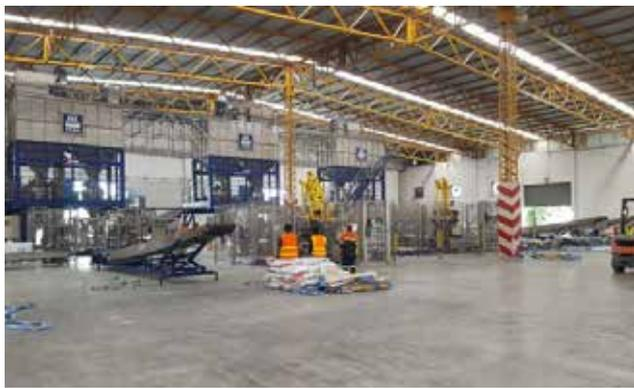
**Figure 1.** 6 x bagging lines for 25 and 50 kg bags installed in three bagging towers with a capacity of 6 x 40 tph.
