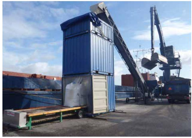
**Figure 4.** Portable triple container set-up at the side of a ship to transfer bulk fertilizers out of the ship into big bags at the key side.
