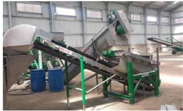
**Figure 5.** Fertilizer screen line to remove bigger particles out of the fertilizers.
