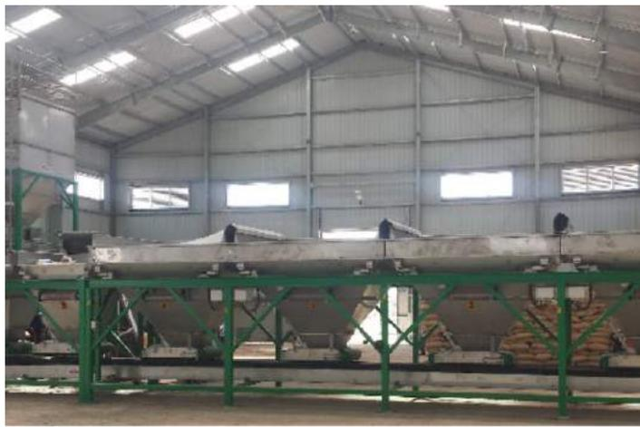
**Figure 4.** Picture of a blender and bagging line in Ethiopia, installed at Bahir Dar with a capacity of 50 tph.
