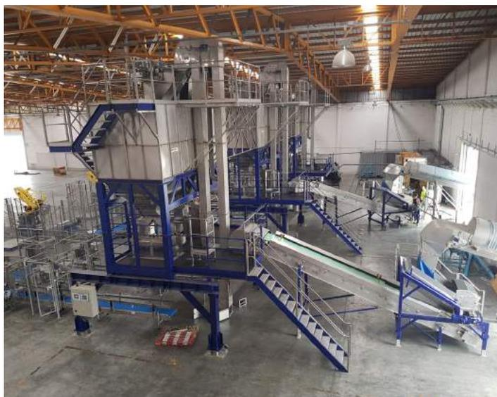
**Figure 5.** Conveyor fertilizer screen with elevator to fill three bagging lines installed at Yara Thailand.
