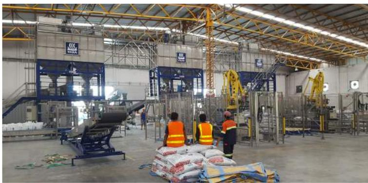
**Figure 1.** EMT Quatro. Three bagging line towers installed at Yara Thailand with two robot stack lines and four conveyors for manual bag stacking. Installed in an existing warehouse with stainless steel hoppers of 20 t each.
