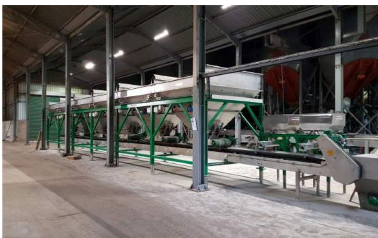
**Figure 2.** Eight hopper Weighcont. Stainless steel Weighcont continuous loss in weight blender with a central production capacity of 100 tph with eight hoppers to blend six raw materials and two micro component products. The machine is in operation at Agron in South Africa.
