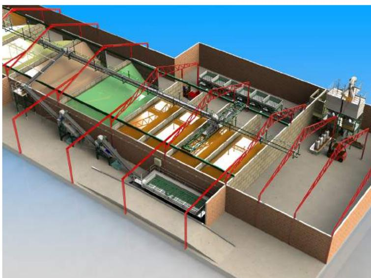
**Figure 3.** 3D CAD impression of a fertilizer storage and blending factory with a product intake conveyor system to fill all boxes equally and a weighcont continuous blender line with two bagging lines: one for small bags and one for big bags. Installed at Agron in South Africa.
