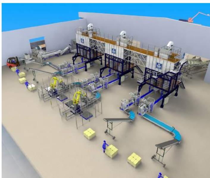
**Figure 6.** 3D Cad impression of Yara's complete factory in Thailand, including conveyor systems and bagging lines.
