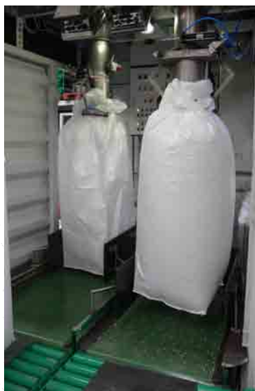
FILLING OF BIG BAGS INSIDE THE CONTAINER
