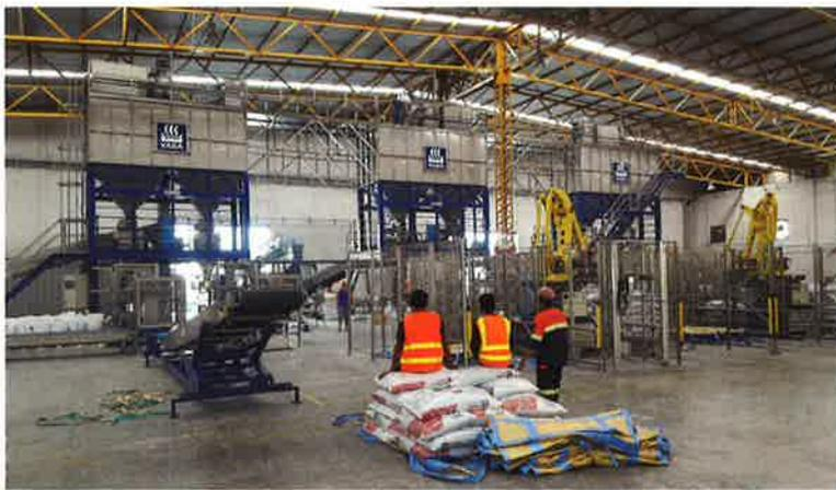
**Figure 4.** EMT small bags filling line with a total handling capacity of 240 tph, installed for a customer in Thailand.
