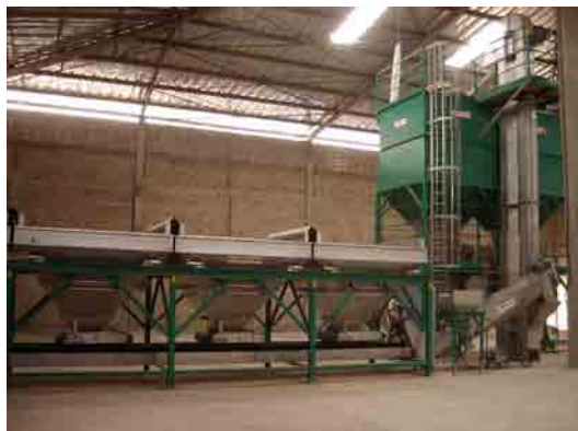
3 hopper Weighcont Blender + Small bag Filling Machine
