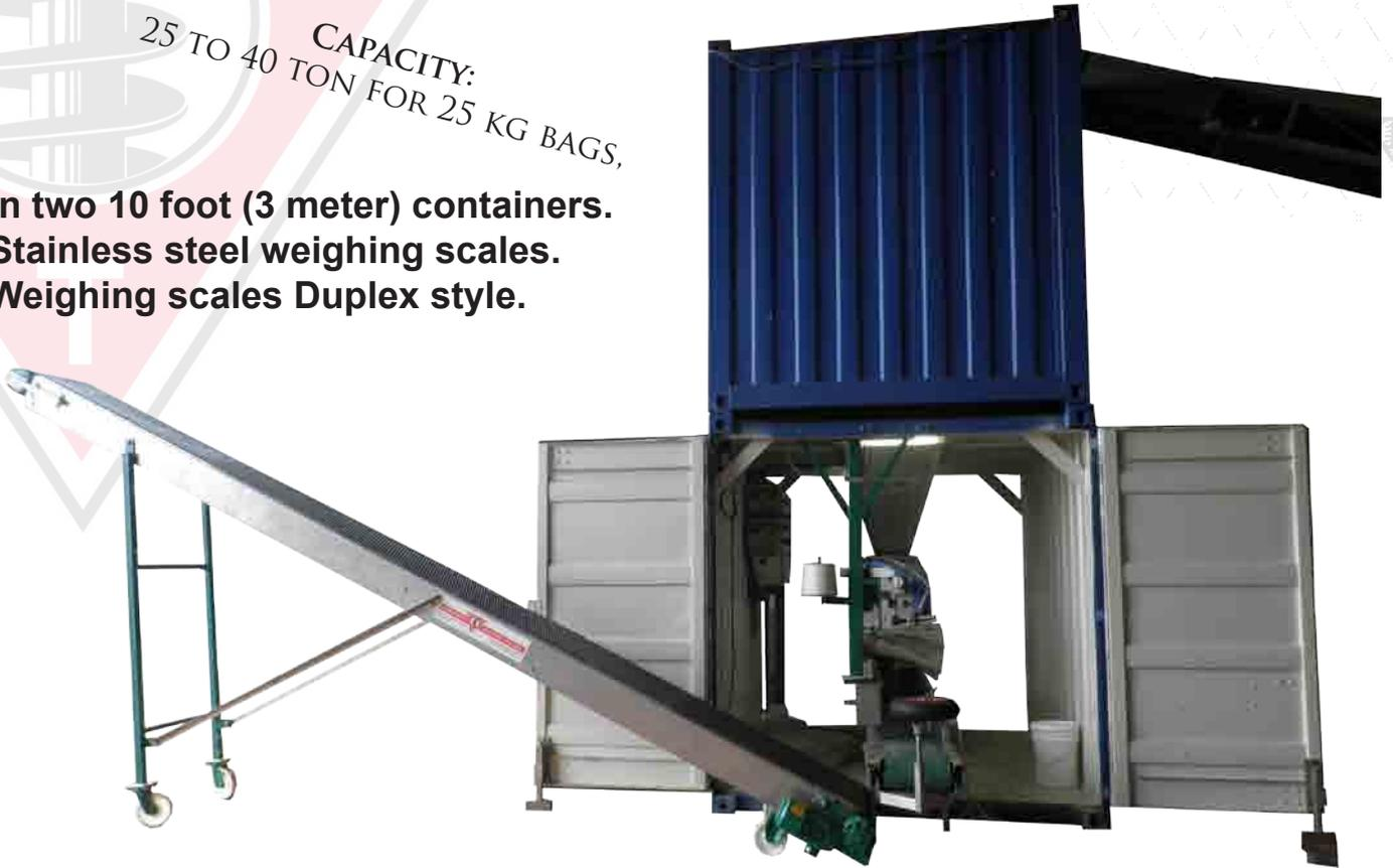
**EMT developed a 20 to 50 kg bag fill line that is completely integrated in 2 normal 10 foot (3 meter) containers.**
